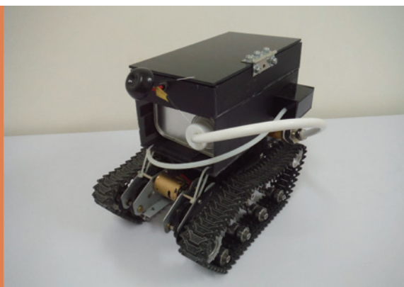
Tracked vehicle equipped with a liquid spraying device
